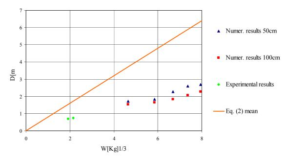
Figure 6: Apparent crater diameter for explosions above the ground level
