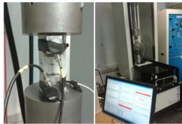
Figure 1: The experimental setup and the AE system
