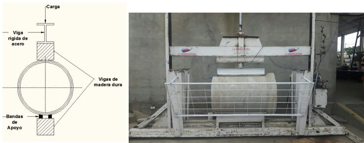
Figure 1: Three edge bearing test set up. Left: schematics cross sectional view. Right: side view.
