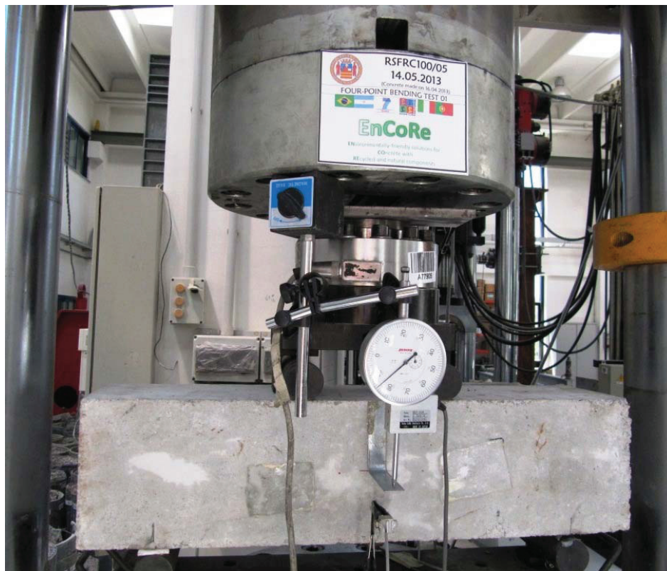
Figure 3: Four-point beam test according to UNI-11039-2 (2003) .
