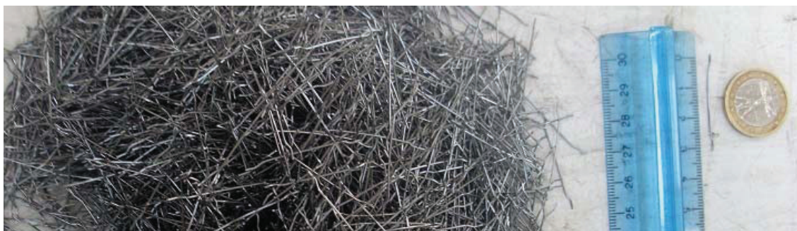
Figure 1: Wirand Fibers FS7 industrial steel fiber.
