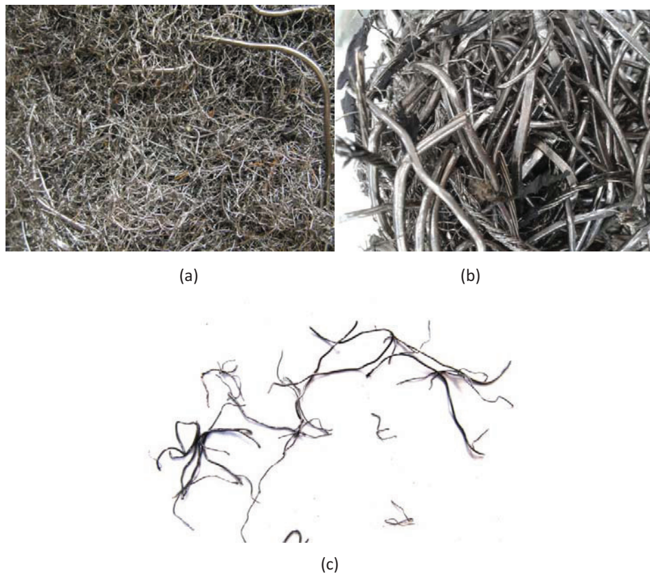
Figure 2: Recycled steel fibers: (a) previous the selection of the coarse pieces, (b) separating the coarse reinforcements and (c) the employed fibers.
