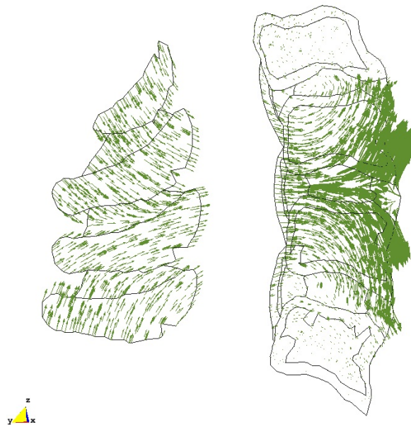
Figure 10: Displacements (x30) of the mid vertical plane due to the forced displacement imposed on the C3-C6 FE model to simulate the discectomy operation.
