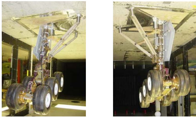
Figure 8: 26%-scale Boeing 777 main landing gear model in the Virginia Tech tunnel.
