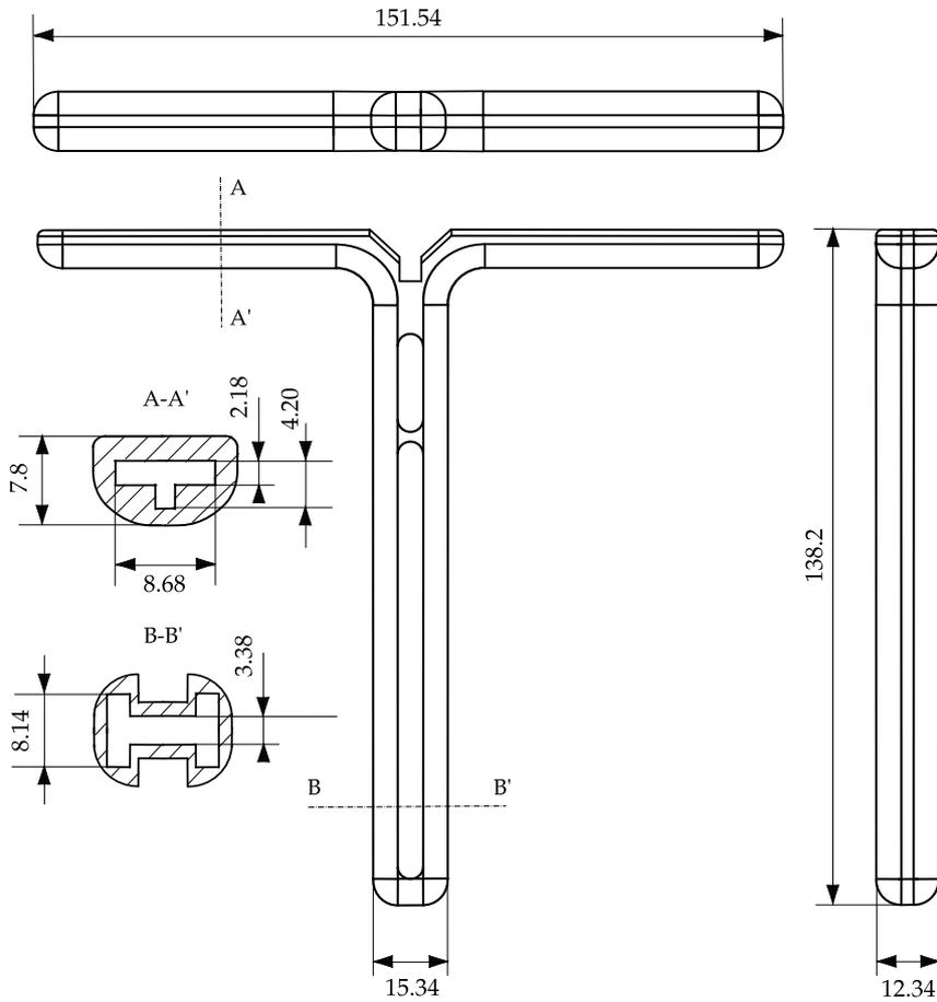
Figure 2: Geometry for CIDR device (dimensions in mm)
