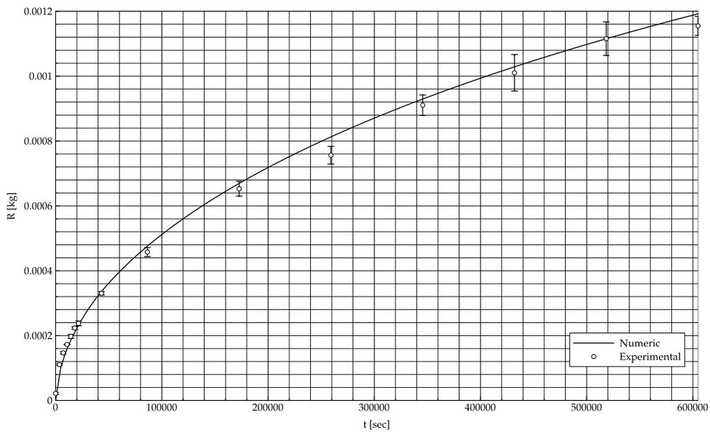
Figure 3: Drug releasing ( $R$ ) along time for analyzed meshes (values accounts for the complete geometry, not a quarter) for 40% of ethanol in the release medium
