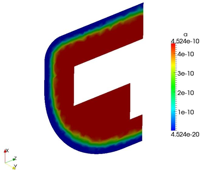
Figure 6: Isovalues of  $a$  for  $t = 7$  days in a transversal cross section
