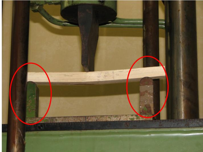
Figure 5: Elasticity test performed on a wooden sample.
