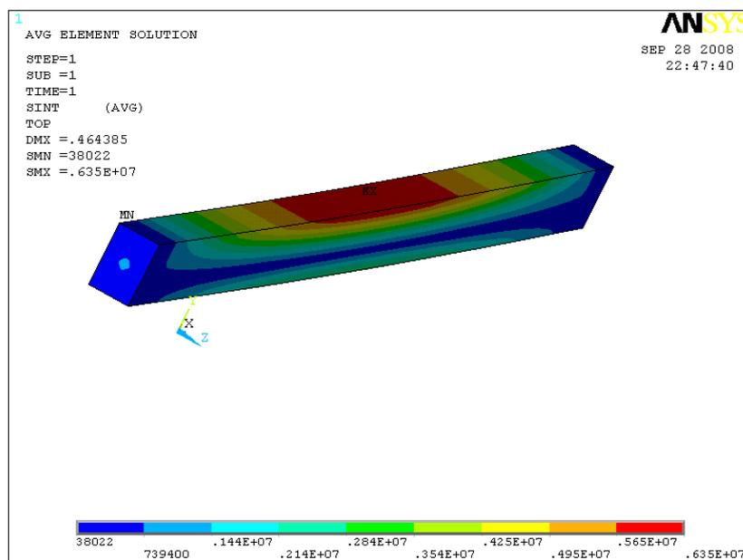
Figure 13: Stress of the wooden beam with a steel T-section profile in relation to the y axis – wooden
