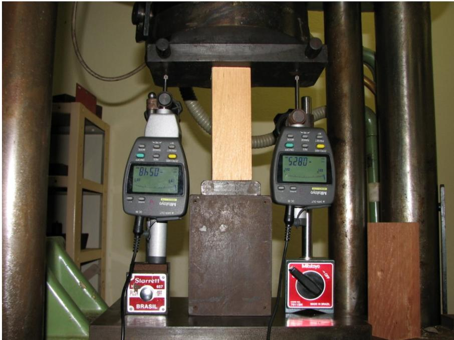
Figure 4: Parallel-to-fiber compression experimental analysis.
