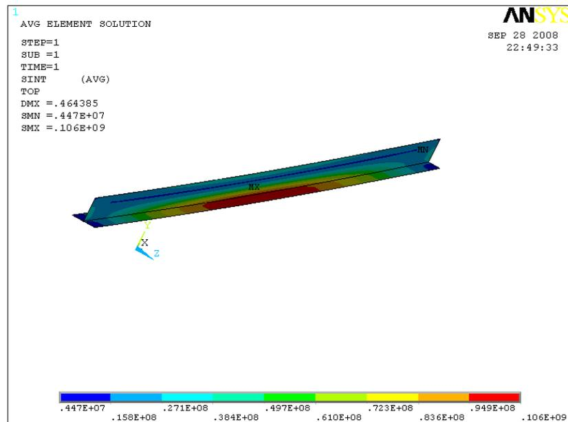
Figure 14: Stress of the wooden beam with a steel T- section profile in relation to the y axis – steel T-section profile.
