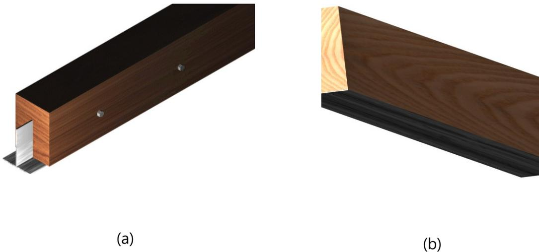
Figure 2: Reinforcement of a wooden beam: (a) with inverted T-section profile; and (b) horizontal surface of the steel plate glued to the underside of the beam in the tractioned region.
