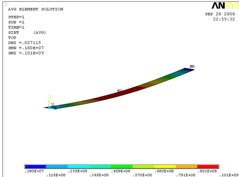
Figure 16: Stress on the Candeia wood beam reinforced with steel plate – steel plate sector.
