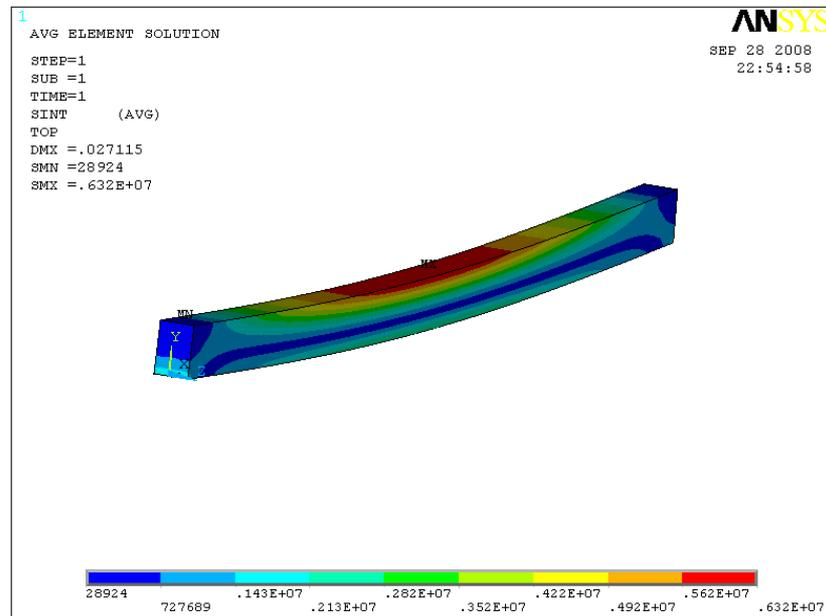
Figure 15: Stress candea-wood beam with steel plate, wooden section.
