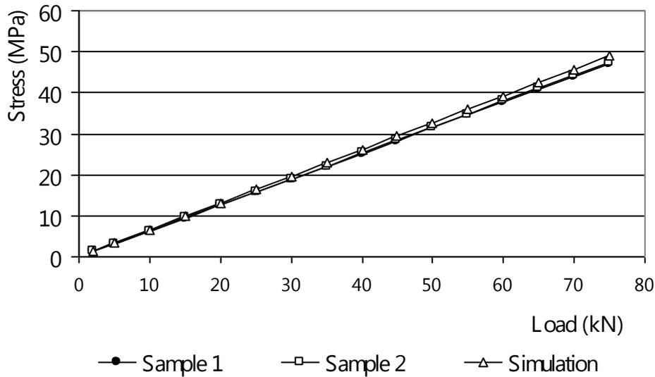
Figure 10: Parallel-to-fiber stress of the two analyzed methods.
