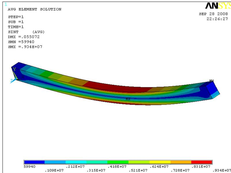
Figure 12: Stress presented by the isolated Candeia-wood beam.
