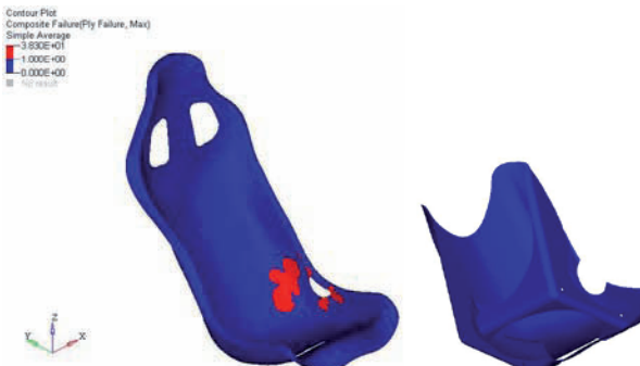
Figure 23: Design 4: Failure index corresponding to the Tsai-Hill criterion on the seat and lower shell.
