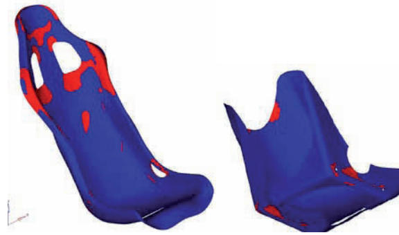
Figure 12: Design 3: Failure index corresponding to the Tsai-Hill anisotropic criterion for the seat and its lower shell.
