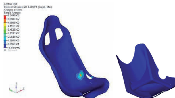
Figure 19: Design 4: Distribution of the maximum principal stress on the seat and lower shell.
