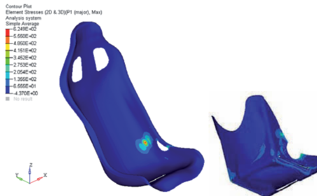
Figure 18: Design 3: Distribution of the maximum principal stress on the seat and lower shell.
