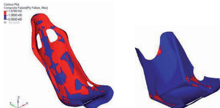
Figure 10: Design 1: Failure index corresponding to the Tsai-Hill anisotropic criterion for the seat and its lower shell.
