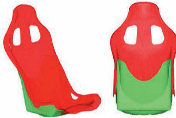
Figure 1: Geometry of the upper (red) and lower (green) parts of the car seat.
