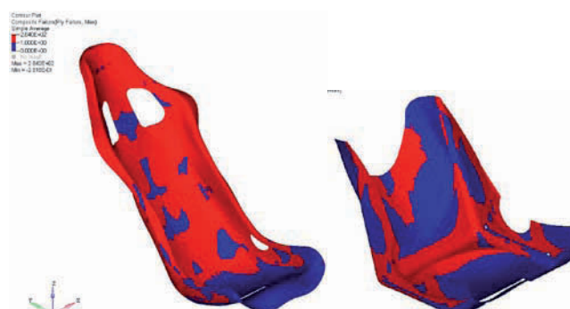
Figure 11: Design 2: Failure index corresponding to the Tsai-Hill anisotropic criterion for the seat and its lower shell.
