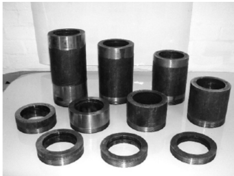
Figure 1: Photograph of mild steel tubes used in the experiments (Jacob et al. 2007).
