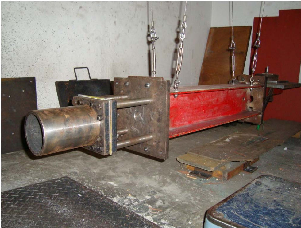
Figure 3: Test rig attached to the ballistic pendulum
