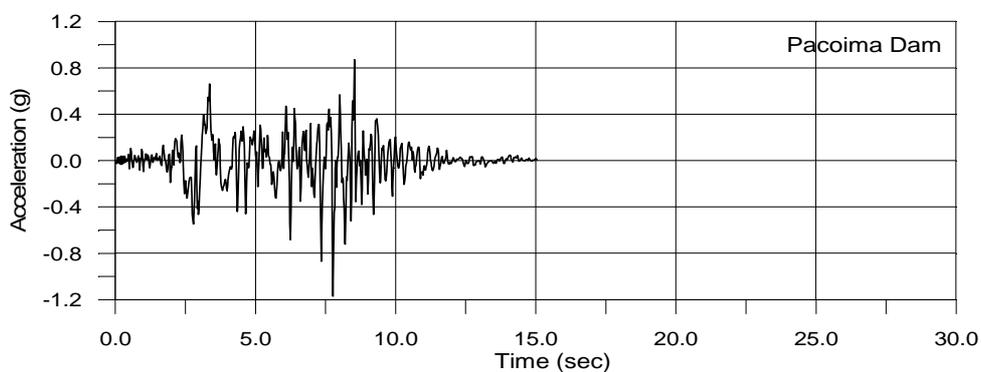
Fig. 2. Acceleration record obtained at Pacoima Dam San Fernando Earthquake 1971.
