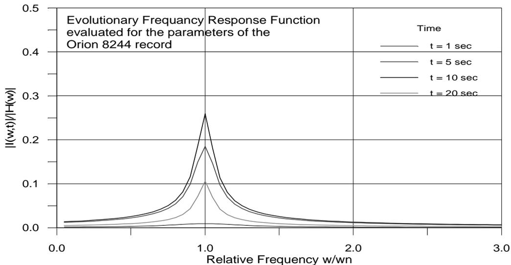
Fig. 9 Evolutionary Frequency Response Function versus relative frequency for the parameters of Orion Radial plotted for different times of evolution.
