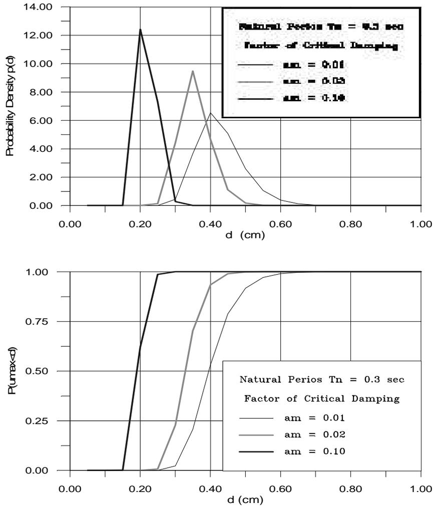
Figure 14. Probability density function and cumulative probability function obtained for a 1DOF structure under the El Centro 1940 record for  $T_n = 0.3$  sec.
