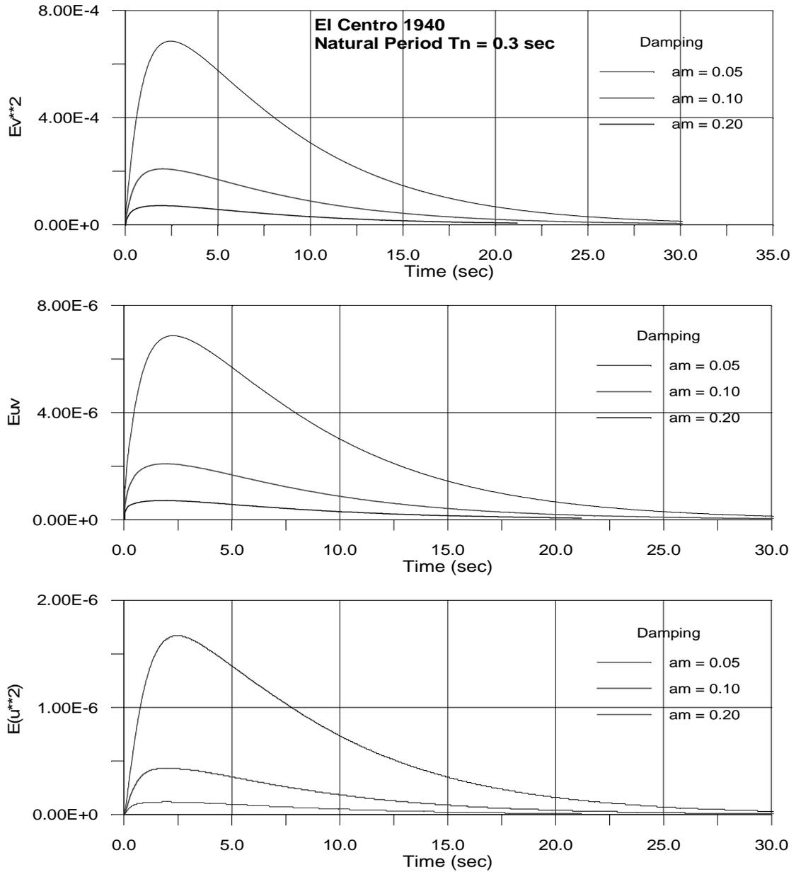
Fig. 11. Square mean value for displacement and velocity and expected value for the velocity displacement product for El Centro 1940 model
