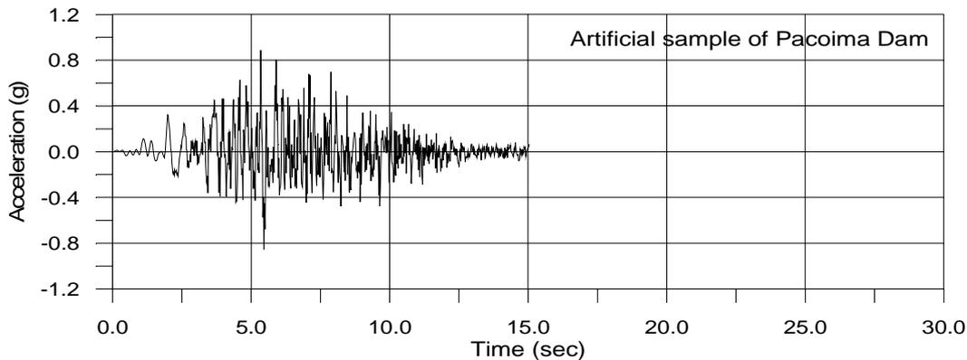
Fig. 4 Artificial sample for the Pacoima Dam accelerogram
