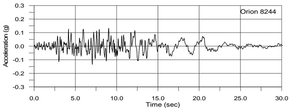
Fig. 1 Acceleration record obtained at Orion 8244, San Fernando Earthquake 1971.
