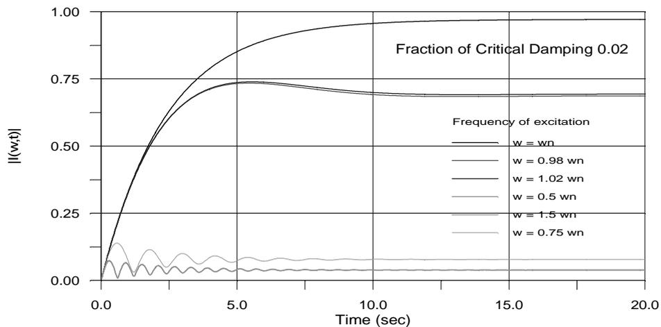
Fig. 5. Evolutionary Impulse Response Function for a step strength function evaluated for a structure with 0.02 of critical damping for different excitation frequencies.
