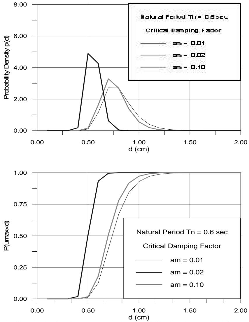
Figure 15. Probability density function and cumulative probability function obtained for a 1DOF structure under the El Centro 1940 record for  $T_n = 0.6$  sec.
