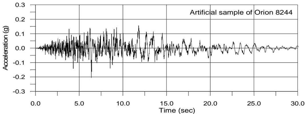
Fig. 3 Artificial acceleration record for the Orion 8244 record
