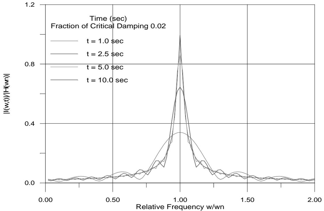
Fig. 7. Function  $I(\omega, t)$  evaluated at different times and as a function of the relative frequency
