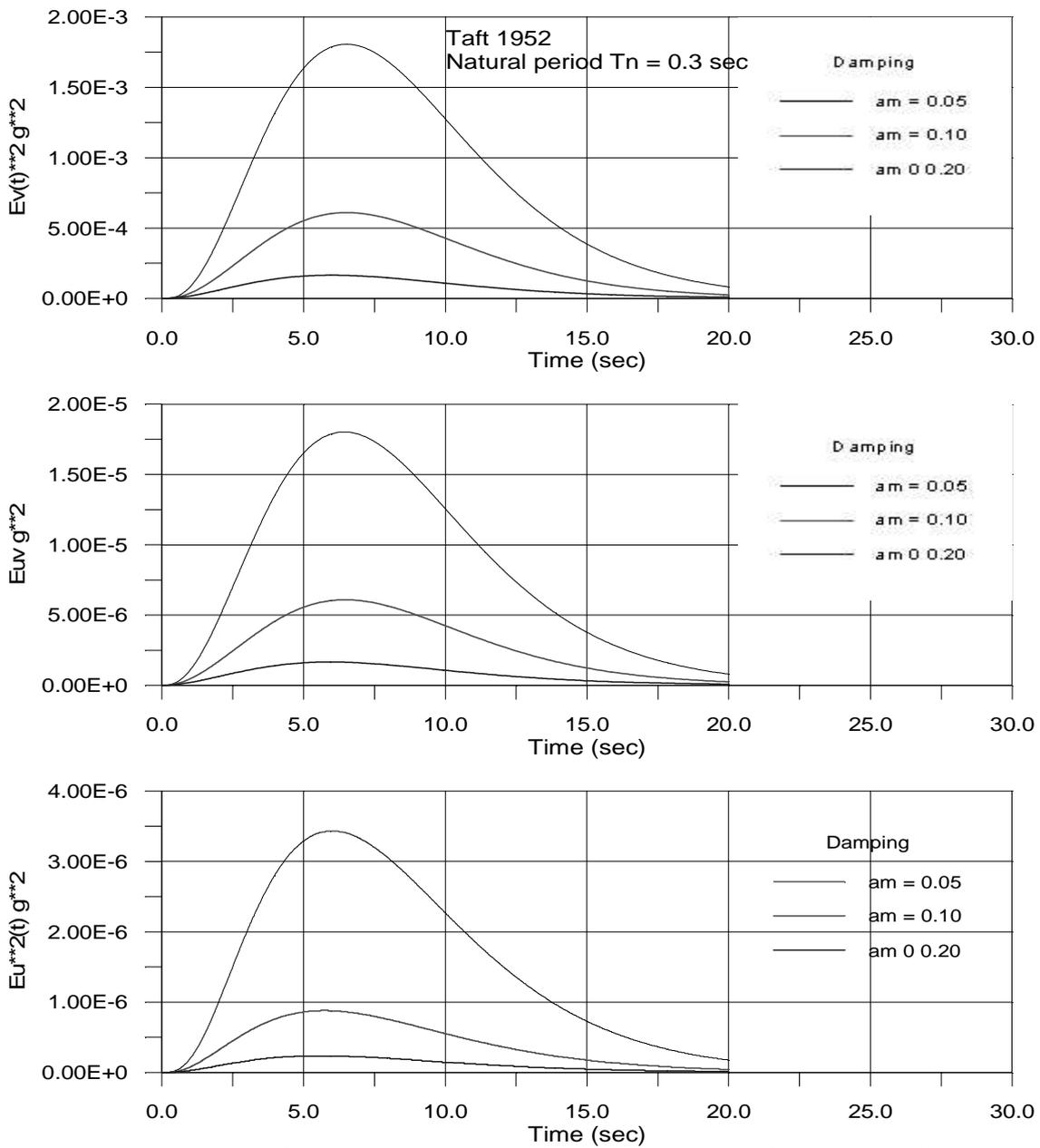
Fig. 13. Square mean value for displacement and velocity and expected value for the velocity displacement product for Taft 1952 model. Natural period of vibration  $T_n = 0.3$  sec
