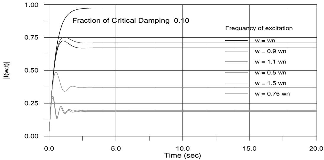
Fig. 6. Evolutionary Impulse Response Function for a step strength function evaluated for a structure with 0.10 of critical damping for different excitation frequencies
