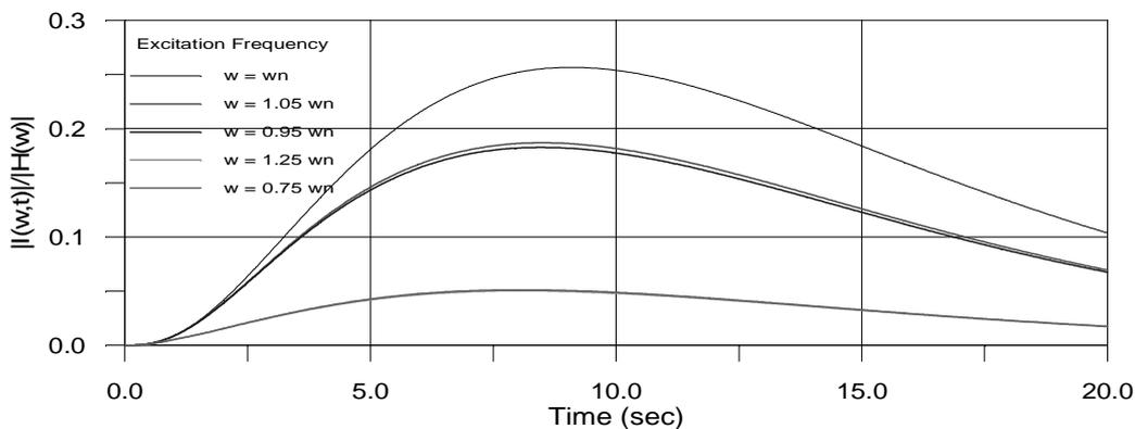
Fig. 8. Evolutionary Frequency Response Function for the parameters of Orion Radial, evaluated at different excitation frequencies.
