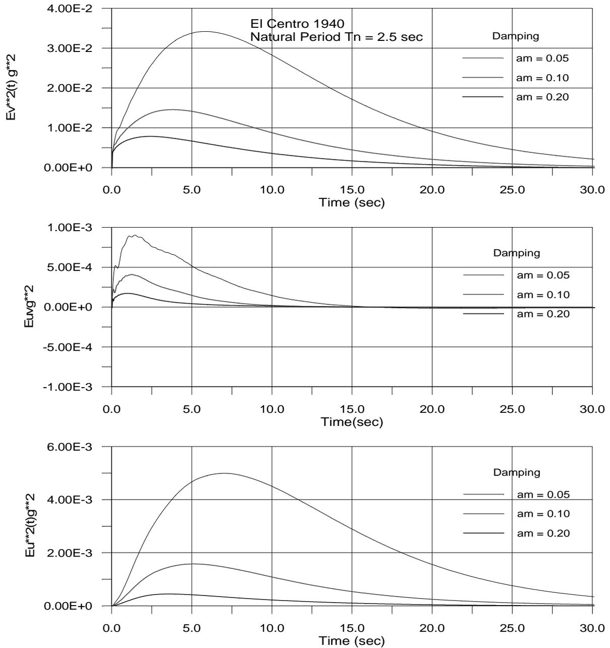
Fig. 12. Square mean value for displacement and velocity and expected value for the velocity displacement product for El Centro 1940 model. Natural period of vibration  $T_n = 2.5$  sec
