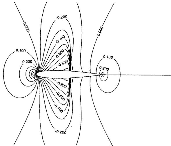
Fig. 5 Pressure contours for NACA 0012, Mach = 0.8 and  $\alpha = 0^\circ$
