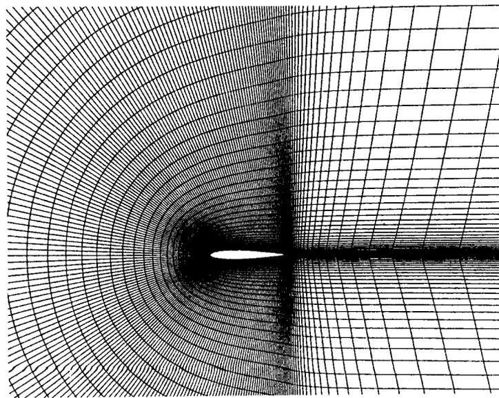
Fig. 4 Grid for NACA 0012, 256x64 cells
