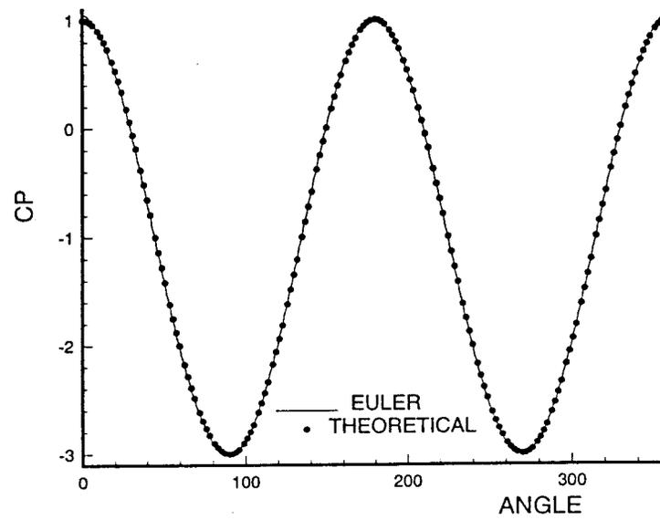
Fig. 3 Pressure coefficient for cylinder, Mach = 0.05
