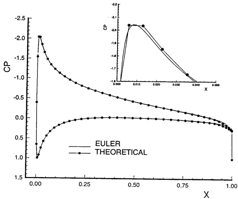
Fig. 6 Pressure coefficient for NACA 0012, Mach = 0.005 and  $\alpha = 5^\circ$
