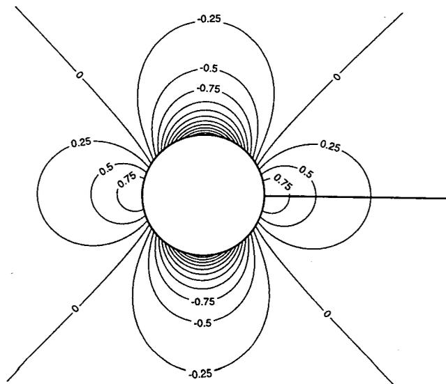
Fig. 2 Pressure contours for cylinder, Mach = 0.05
