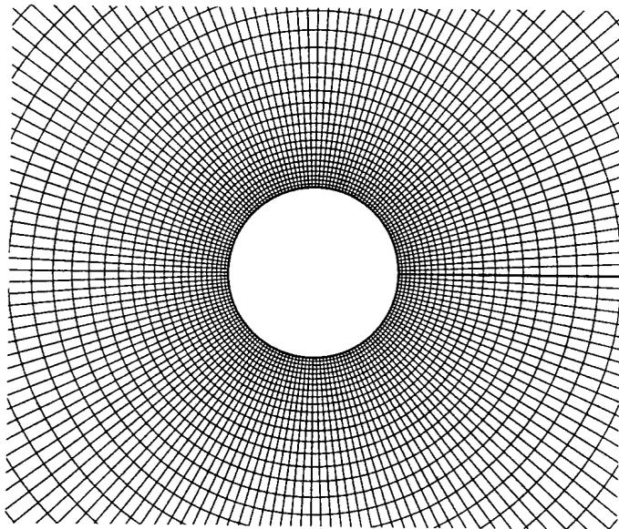
Fig. 1 Grid for cylinder, 160x48 cells
