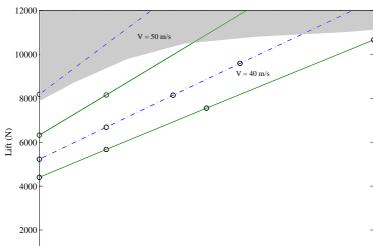
Figure 4: Lift force as a function of angle of attack. Results for the flexible wing are shown as solid lines and the corresponding results for the rigid wing are shown as dashed lines. The shaded area is the region of dynamic instability (flutter) for the flexible wingsle of Attack (deg)
