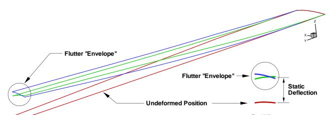
Figure 6: Depiction of the fluttering wing. The extreme positions of the wifigd Hier a typical flutter response are shown superimposed on the undeformed wing position.
