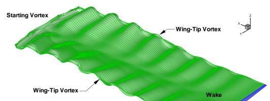
Figure 2: Aerodynamic representation of a flexible wing and the wake that trails it during a stable aeroelastic response to an impulsive start.
