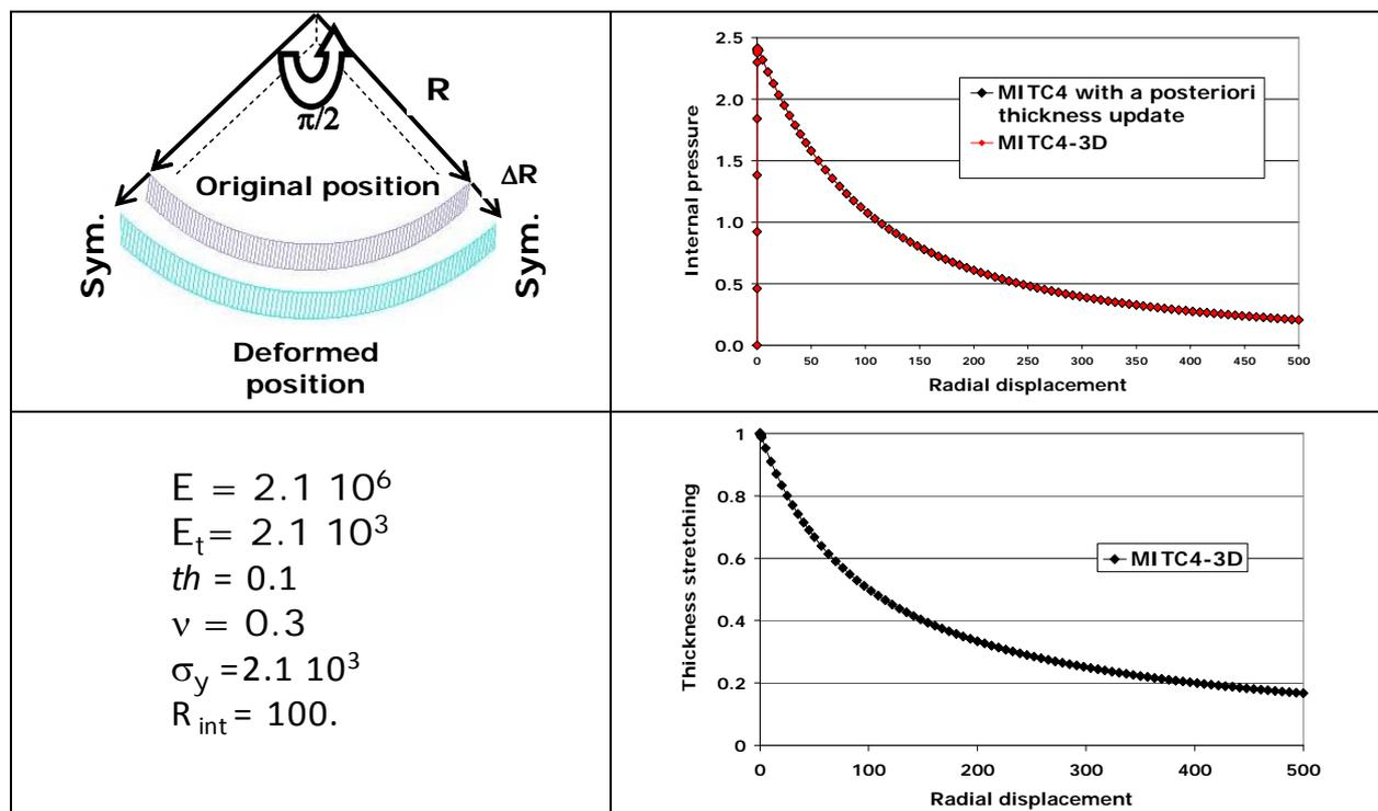
Figure 3: Inflation of an infinitely long elasto-plastic cylinder
