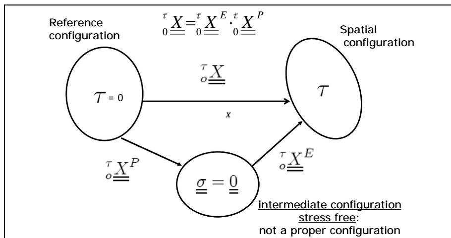
Figure 1: Lee's multiplicative decomposition of the deformation gradient
