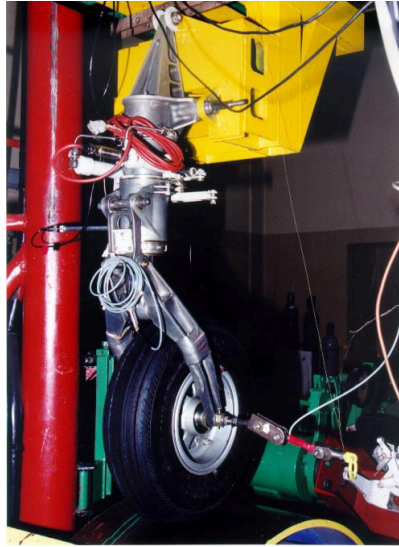
Figure 3: A gear landing during the test
